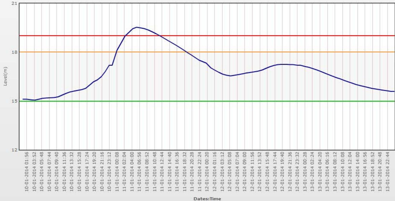
■ danger level   ■ alert level   ■ normal level   ■ water level
