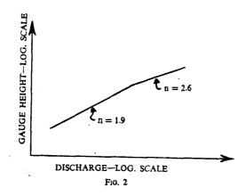
(b) breaks in the rating curve also occur where controls become effective e.g. a constriction in the channel downstream of the gauging site may serve as a control from medium to high stages only; during these stages the equation may not apply, or if applicable, have a changed value of n (see Fig. 3);
