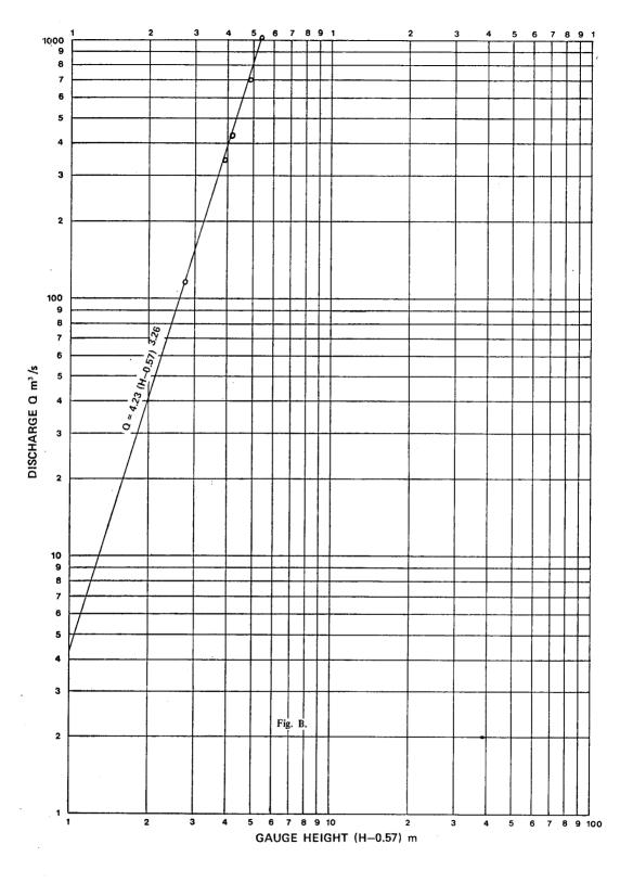
The values of n and K can be determined also graphically from Fig. B. The intercept of the straight line on the vertical axis gives K = 4.23, while the slope (tangent of the angle which the straight line makes with the horizontal axis) gives n = 3.26.
